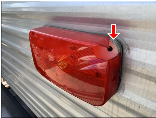
(2) Inspector observed that the tail light lens on the rear curbside is broken.
